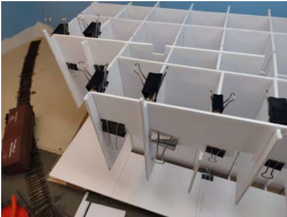
Lots of corner bracing to keep the warehouse square.
