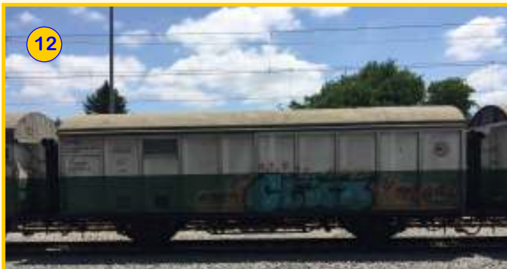
One of the cars in the weed-spraying train, converted from an old four-wheel box car. Note the diaphragms connecting the cars.
