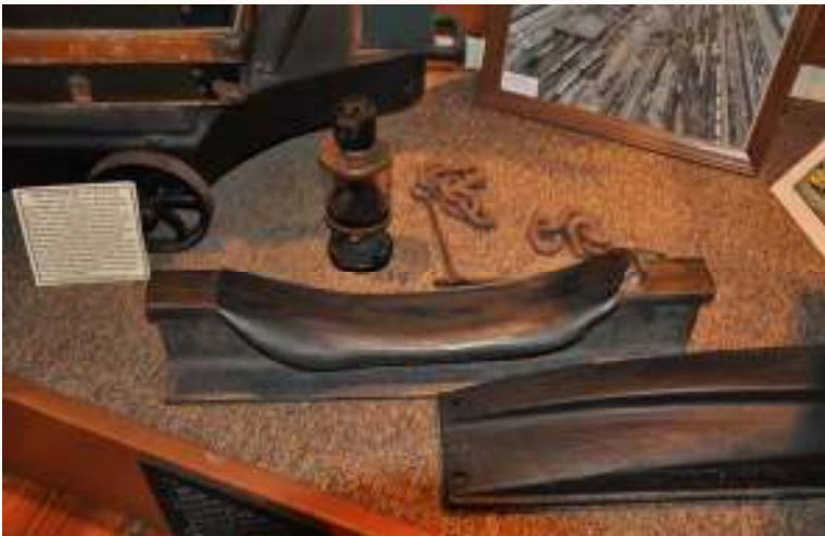
Display of a section of melted rail caused by a malfunctioning traction motor on a diesel engine. One axle spun at high speed on an otherwise stationary engine. Friction caused the wheel to melt the underlying rail in less than a minute.
