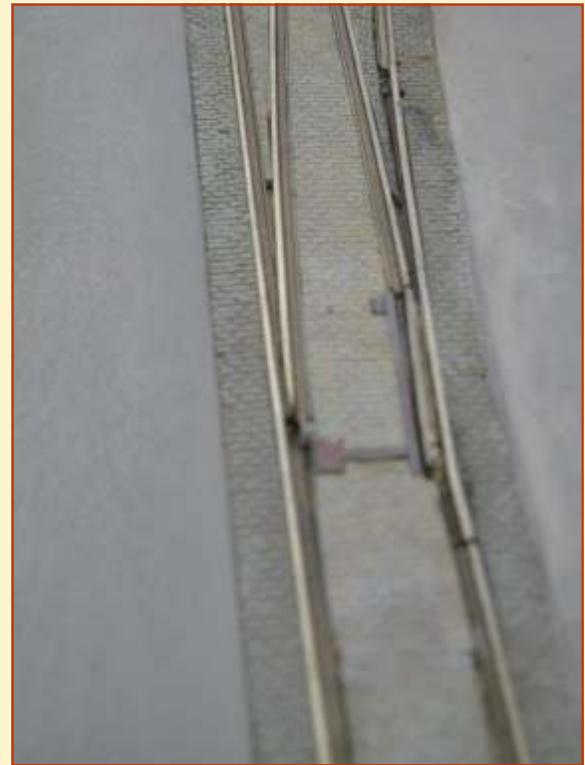
Operating single point switch using the street trackage on Carroll Street (yes, it does work properly)
